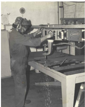
Profile cutting - Grasshopper blade holders en50b plate
